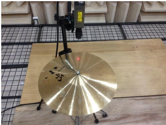
Fig.5 - Measure the surface vibration velocity
